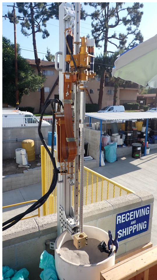
3-meter drill stem testing in lunar simulant
