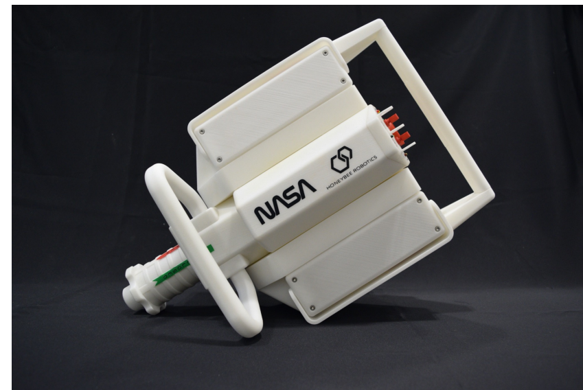
3D printed mockup for human factors testing
