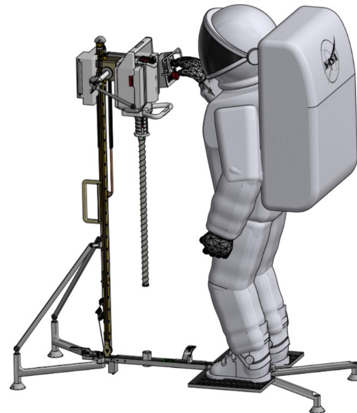
Astronaut Lunar Drill (ALD) Multipurpose drill to obtain drill cores down to 3 meters
